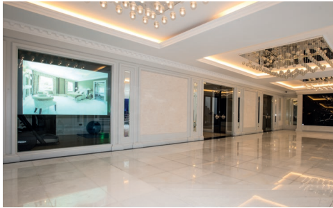
Electronic privacy glass creates a projection screen.
